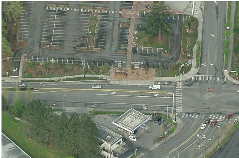
FIGURE 4.4: Bus Shelter and Bus Pull-Out Located on the Major Roadway (Source: Bing.com/maps)
