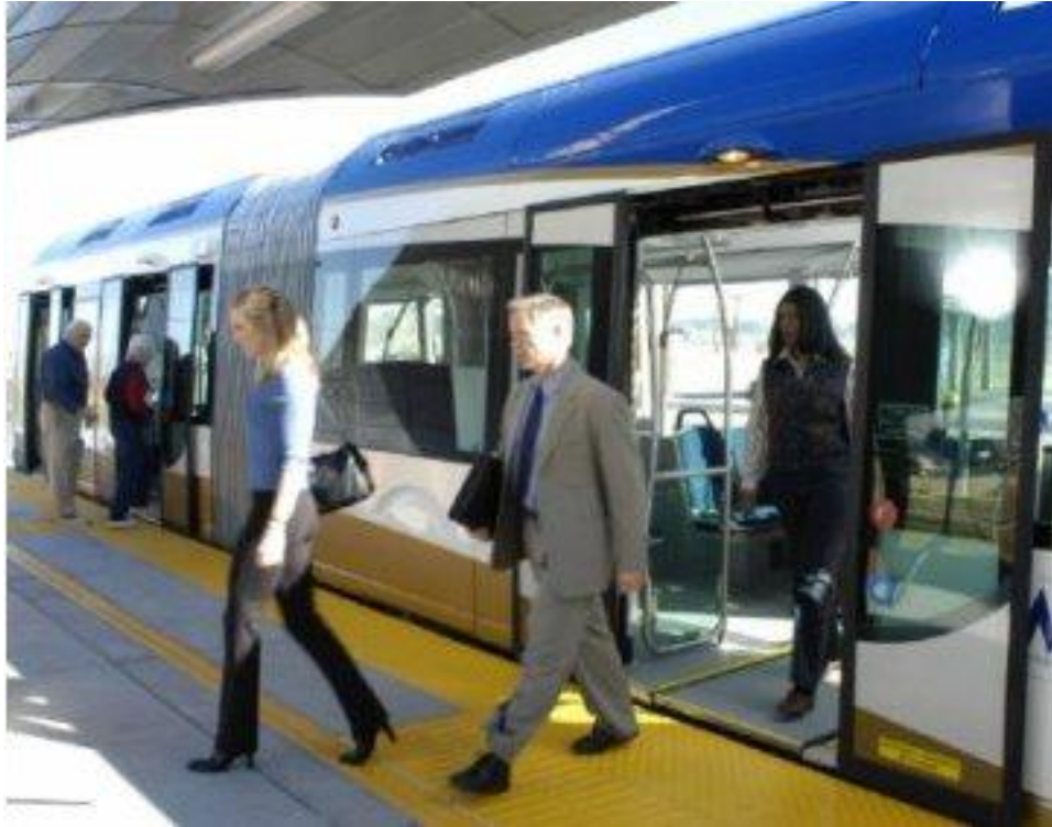
FIGURE 4.14: Passengers Boarding and Alighting a Las Vegas MAX Low-Floor Vehicle (Source: tstc.org)
